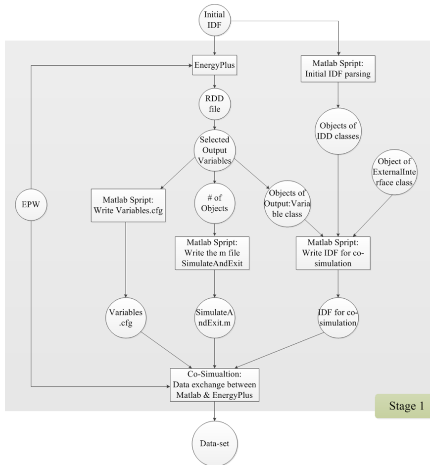
Figure 23: Stage 1 – Select objects — output variables of EnergyPlus — and run a simulation to receive simulated results
